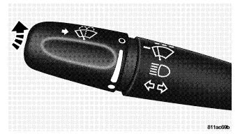
The wipers and washers are operated by a switch in the multifunction control lever. Turn the end of the handle to select the desired wiper speed.
